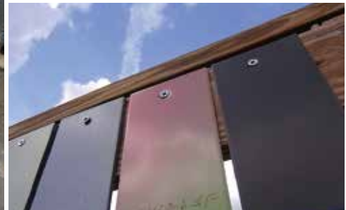
Natural exposure test in Japan & South Florida, USA
